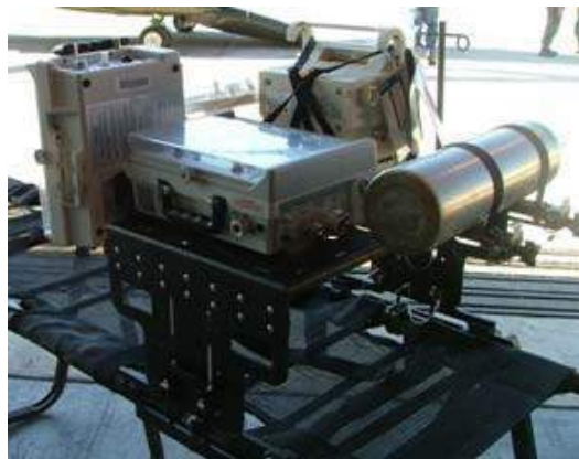
Figure 3: Special Medical Emergency Evacuation Device (SMEED) Attached to Litter and Outfitted with Patient Monitor, Ventilator, Suction Apparatus, and Oxygen Cylinder.
